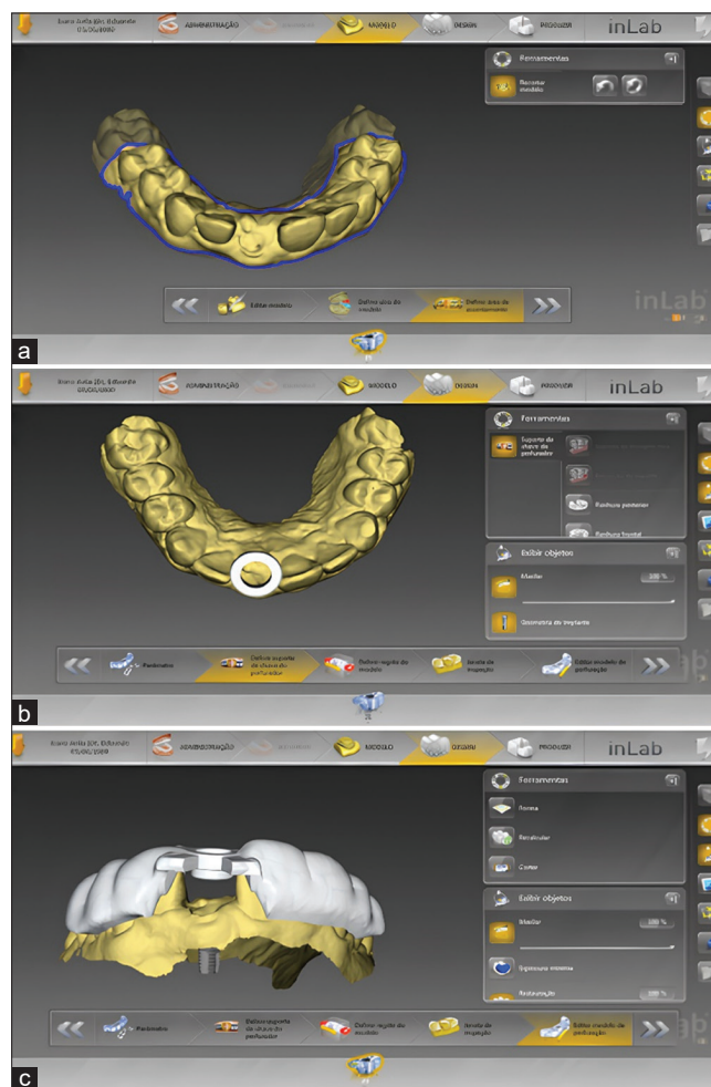
Fig. 3: (a) Definition of the limits of the surgical guide. (b) Ring position. (c) Projection of the final surgical guide Reprinted with permission from Mukai et al. [29]
