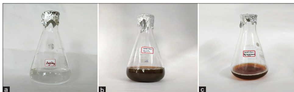
Fig. 2: Visual observation of silver nanoparticles synthesis (a) AgNO 3 solution, (b) color change on the addition of piper betel stem aqueous extract, (c) silver nanoparticles with 1% chitosan
