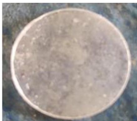
Fig. 6: KBr pellets of transmission in infrared spectroscopy
