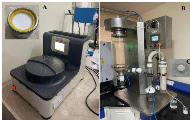
Fig. 1: IBR-NS developed using ball mill (A) followed by spray dryer technique (B) and spray dried product (C)
