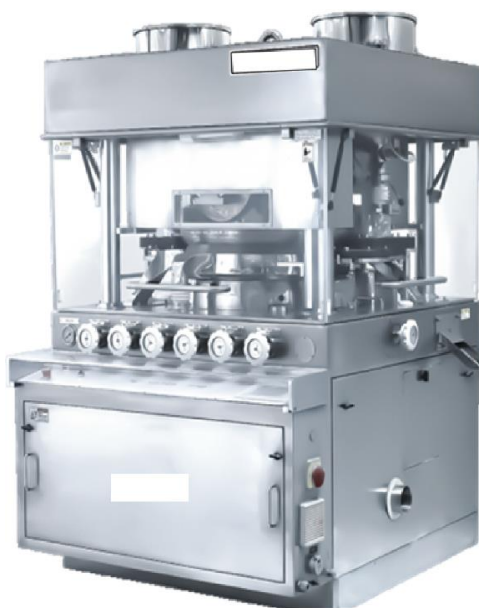
Fig. 7: Double-sided tablet press showing simultaneous compression of two powder layers from both sides, enabling the formation of bilayer tablets with distinct layers for controlled drug release [56]** https://www.fluidpack.net/blogs/b4-double-sided-rotary-tablet-press-features-and-applications
