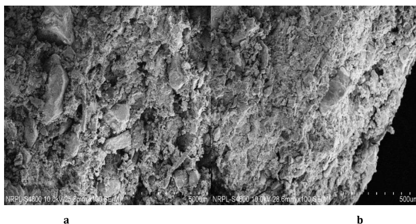
Fig. 4: a. Scanning electron microscopy image of F7 trial batch (drug loaded, prepared by direct compression) with processed poultry egg shell powder as matrix base at 5000 x determined by Hitachi S4800, b. Scanning electron microscopy image of F8 trial batch (drug loaded, wet granulation) with processed poultry egg shell powder as matrix base at 5000 x determined by Hitachi S4800
