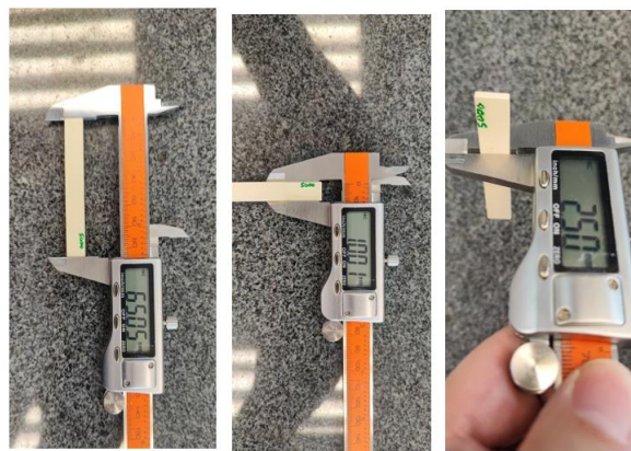
Fig. 4: PEEK sample size for flexural strength test
