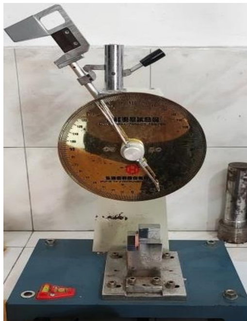
Fig. 3: Charpy impact testing machine (HT-8041B Charpy impact testing machines hung Ta taiwan)
