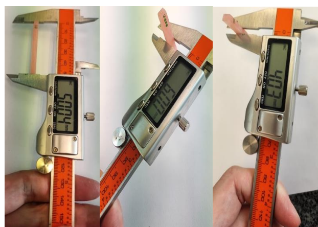
Fig. 7: PMMA sample size for impact strength test
