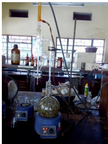
Fig. 1: Steam distillation of C. citratus and O. gratissimum essential oils using the clevenger apparatus
