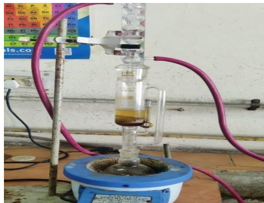
Fig. 1: Extraction of dried roots and rhizomes of liquorice using soxhlet apparatus
